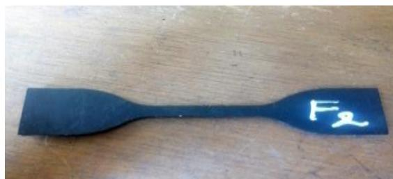
Figure 2. Tensile test sample of a HDPE-porcelain mixture after shaping in the injection molding machine
