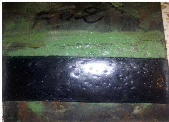
Figure 1. Three-layer coating on a metal substrate
