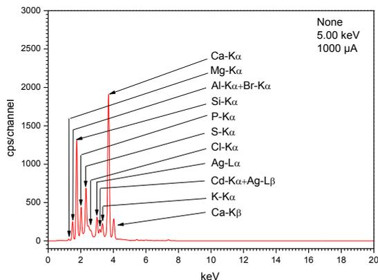
**Figure 4.** XRF spectrum of sludge of Guelma wastewater treatment plant achieved without a filter, 5.00 kV and 1000 μA.
