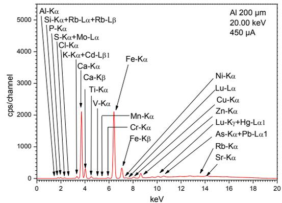
**Figure 2.** XRF spectrum of sludge of Guelma wastewater treatment plant achieved with an aluminum filter of 200 μm thickness, 20.00 keV and 450 μA.
