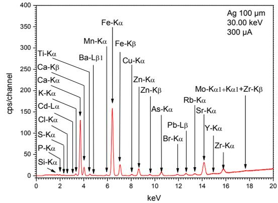
**Figure 1.** XRF spectrum of sludge of Guelma wastewater treatment plant achieved with a silver filter of 100 μm, 30.00 keV and 300 μA.
