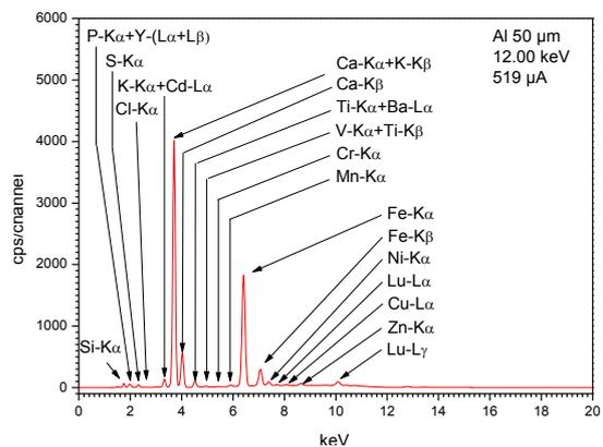
**Figure 3.** XRF spectrum of sludge of Guelma wastewater treatment plant achieved with an aluminum filter of 50 μm thickness, 12.00 keV and 519 μA.
