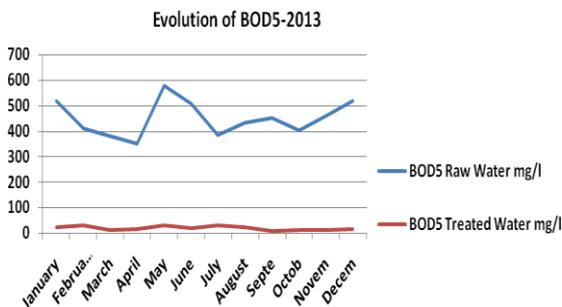
Figure 3. Graphic representation of the evolution of BOD<sub>5</sub> to the inlet and the outlet of the WWTP.
